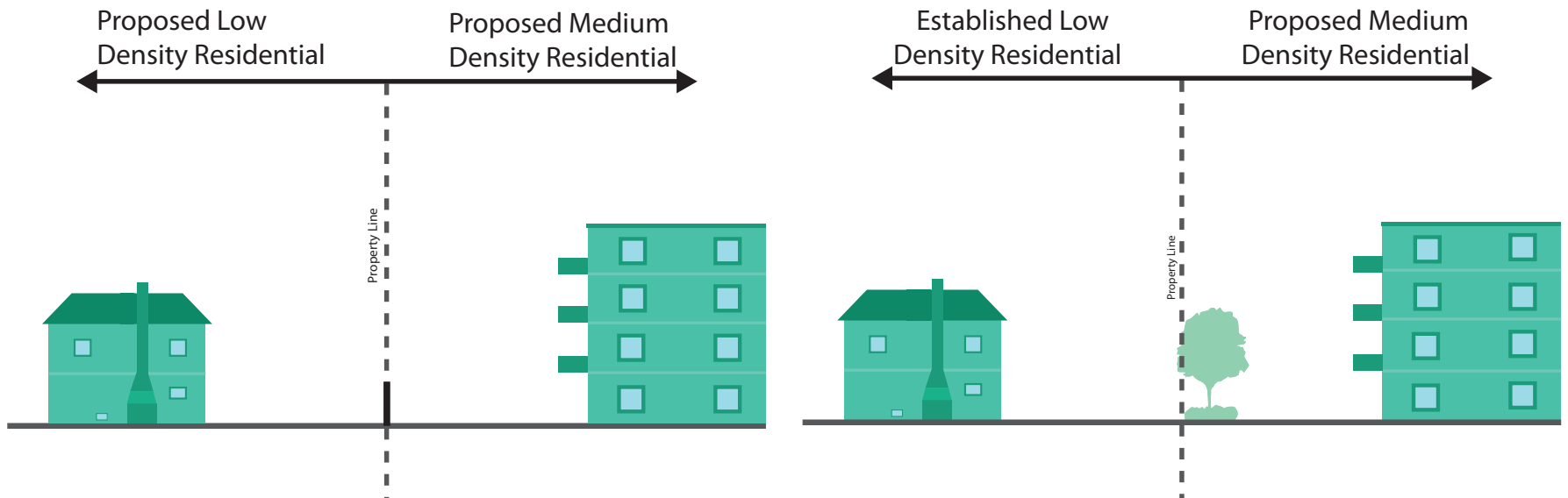
Example of Medium Density Residential uses maintaining a 45 degree angular view plane from proposed and established Low Density Residential Areas
